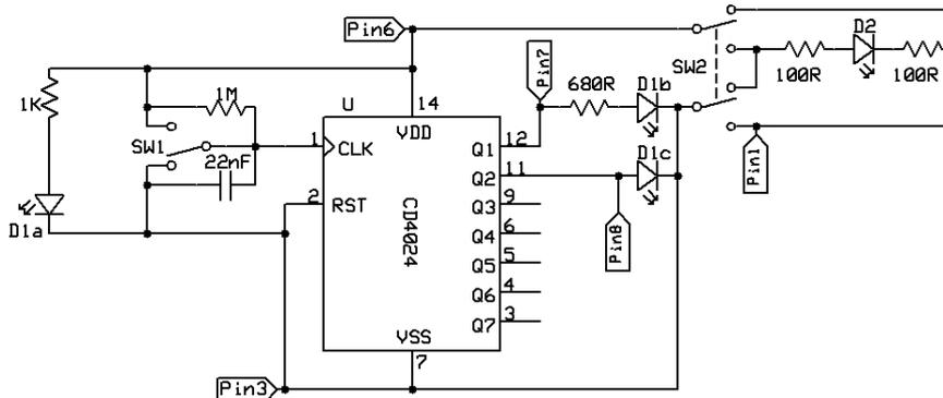
1K and 680R resistors helps adjust the brightness of the tri-color LEDs. Adjust to taste. The 100R resistors prevent pulling pin 1 below 3.3V
